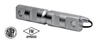
This product is designed for use in industrial and out-door environments. Nickel plated steel construction limits corrosion from outdoor use. The IP67 sealing makes it suitable for applications that are subject to high-pressure wash down. Tank weighing is made simple when this load cell is combined with the EZ mount mounting hardware it was designed for. Its high accuracy and availability in high capacities make it ideal for certified truck and rail scales.
